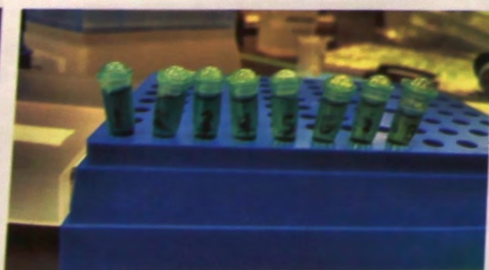
Phosphate Standard developing with Malachite Green Reagents
